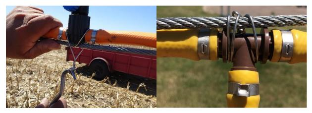
Above you can see how the adaptor tee and tee are secured to the cable
